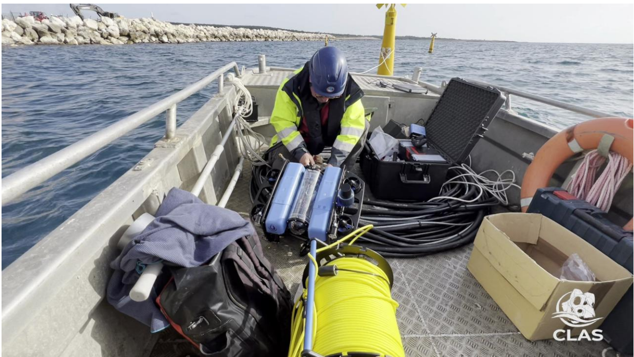
A CLAS inspector prepares the ROV for the inspection of the EDF Martigues power station seawater intake structures.
